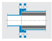
A weld-on counter flange with larger bolt circle diameter on the unlined pipe is a proven solution to connect pipes.
