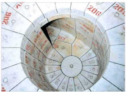
Wear protection for high temperatures involves problems due to thermal stress between the outer steel component and the rigid lining. These problems can be solved by using KALCOR as wear protection material and the right mechanical fixing method: bolted connections or welded steel inserts. Example: drying drum in a chemical plant at 800 °C / 1.472 °F.
