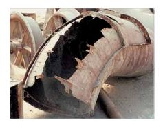
The transport of bulk materials in many basic industries and in coal fired power stations is associated with heavy wear of the system components Not only is the original equipment investment lost, plant shutdowns and production losses combine to destroy the capital base of the company.
