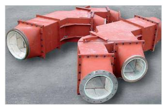
Pulverized coal distributor boxes protected with KALCOR for large surface lining and KALOCER to offer maximum wear resistance
