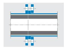
Lined pipes can be connected to each other easily with a fixed collar and a loose turnable flange on one end.
