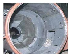
Cyclone used in a soil decontamination system – effectively protected with KALMETALL-C
