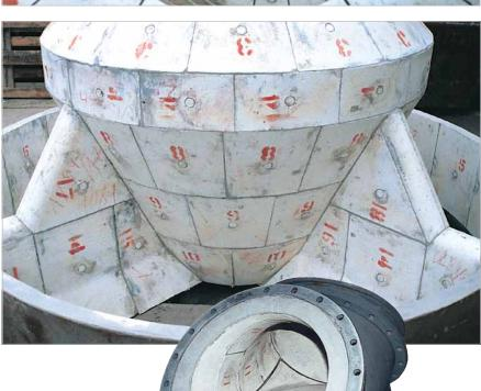
KALCOR bend with special deflectors to distribute the conveying stream of coal
