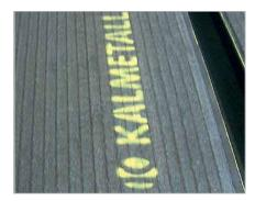
Hard overlay welded standard plates
