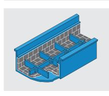
Typical system components with wear protection lining
