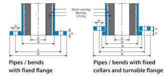
**Designation of pipe bend:** Inside diameter (d) 60 mm, radius (r) 1,000 mm, angle (a) 90° as defined in Kalenborn company standard Rd 6a:
