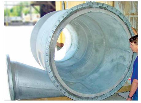
Pulverized coal distributor made of KALSICA-N installed in a power station
