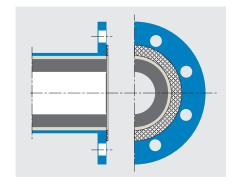
ABRESIST pipe with a fixed flange
