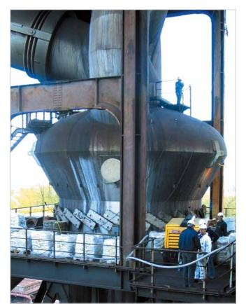
Separator of a cement mill lined with KALCRET-BNX, up to 3,200 mm diameter
