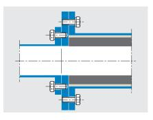
Unlined pipes, pumps or fittings can be connected with a lined pipe using an adapter flange.
