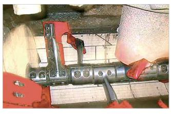
Drum mixer for concrete lined with KALOCER high alumina ceramics; mixer tools made of KALMETALL-C hard casting and/or KALEN-PU plastics
