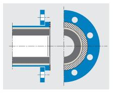
ABRESIST pipe with a fixed collar and turnable flange
