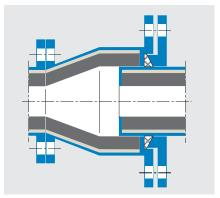
Expansion joints in a hydraulic bottom ash pipeline
